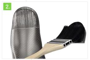
Apply a thin film of contact adhesive, suitable for TPU material. Then, leave to air dry.
